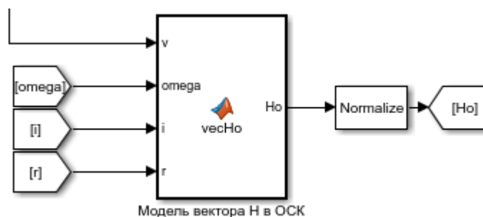
Fig. 19 Block for simulating the Earth's magnetic field
