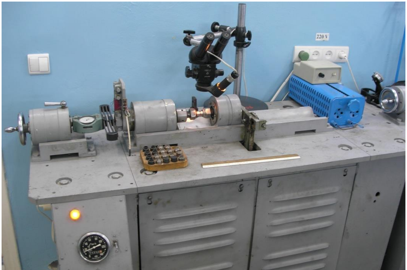
Figure 2.1 - General view of installation MFK-1 for testing the fretting
