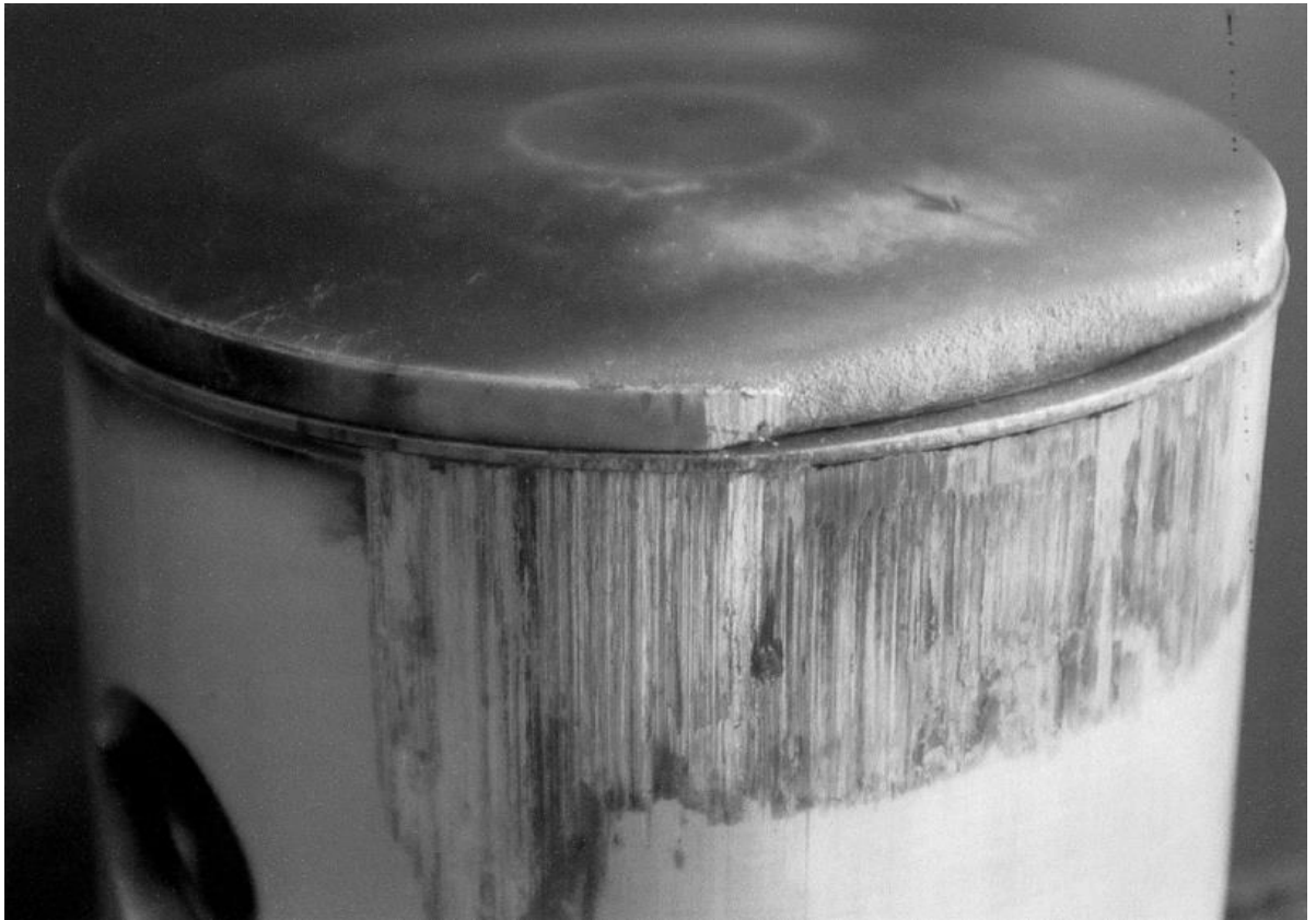
Figure 1.2 - Eized piston from combustion engine
