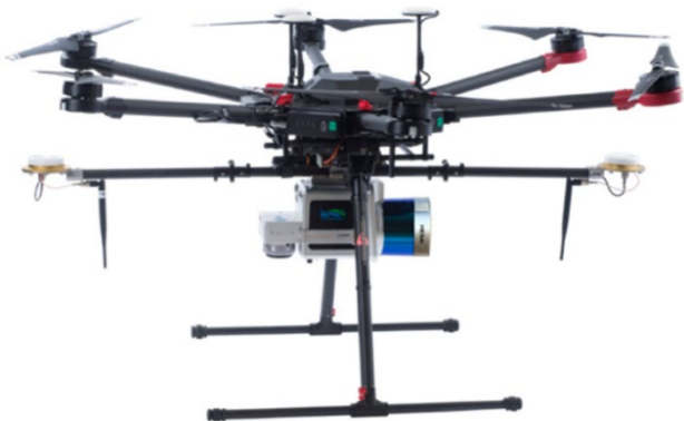
Picture 2. Faster R-CNN fined mine. Picture 3. Prototype of adrone used for high-resolution image capture
