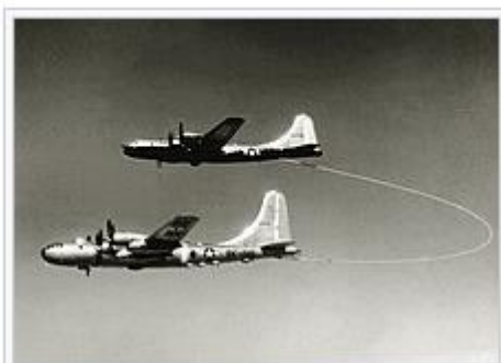
The US Air Force Boeing B-50 Superfortress Lucky Lady II being refueled by grappled-line looped-hose during the first non-stop circumnavigation of the world by air (1949)
