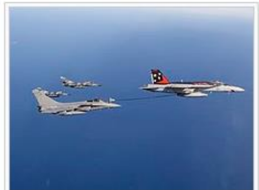
An F/A-18E Super Hornet of the US Navy acts as a buddy tanker for a Rafale of the French Navy over the Arabian Sea, 2015
