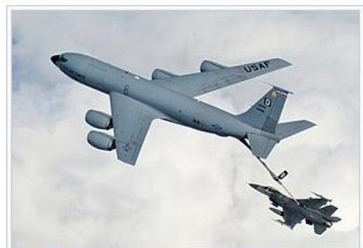
A KC-135 Stratotanker refuels an F-16 Fighting Falcon using a flying boom
