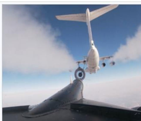
Tu-95M filling rod and filling cone from Il-78M aircraft
