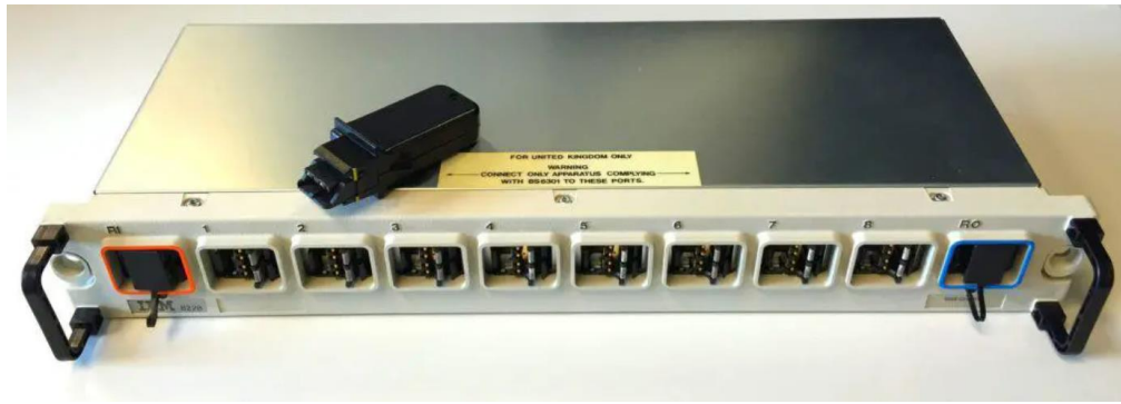
Рис. 1.1. IBM 8228 Multistation Access Unit
