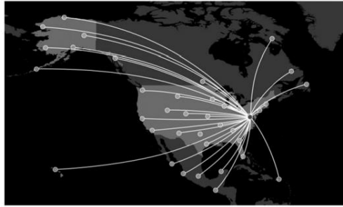
Figure. 2.15. WAAS showing links between reference receivers and the East Coast WAAS master station.
