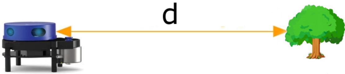
Fig. 3.2 Calculation of the distance from LIDAR to the object
