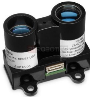
Fig. 3.5 Appearance of LIDAR-Lite 3 Laser Rangefinder
