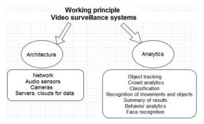
Fig. 2. Components and functionality of the video surveillance system
