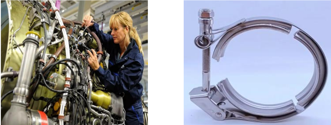
Figure 1-1 Piping System in a modern aircraft engine and Pipe Clamp
