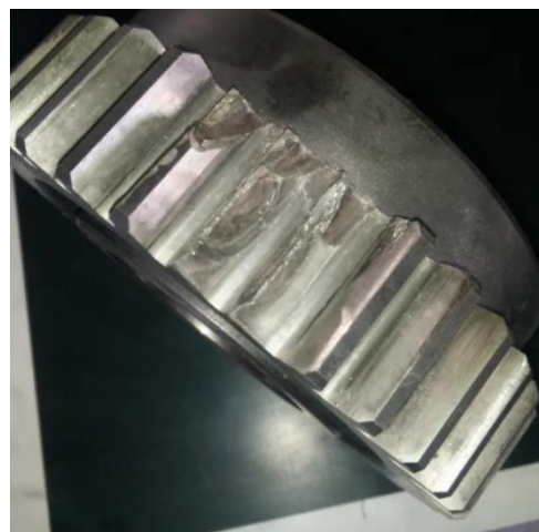
Figure 1.2 - Gear with broken teeth
