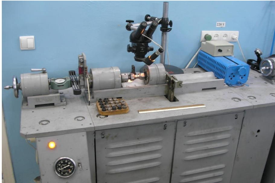
Figure 2.1 – General view of the MΦK – 1 installation for the testing on fretting
