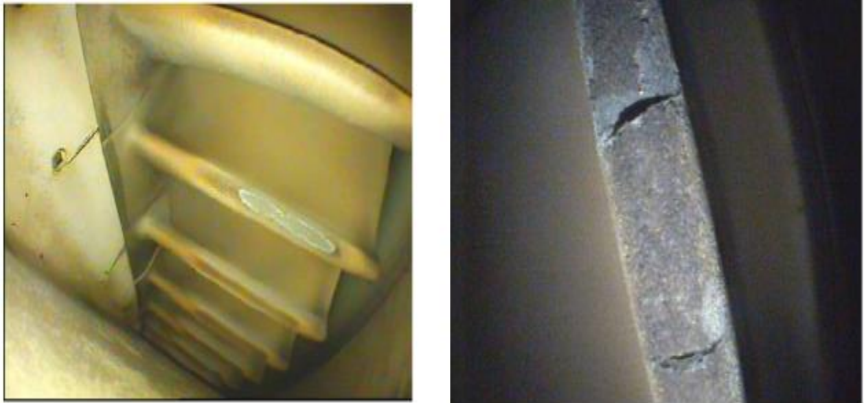
Figure1.10 – Exemplary types of thermal damages to leading edges of turbine rotor blades
