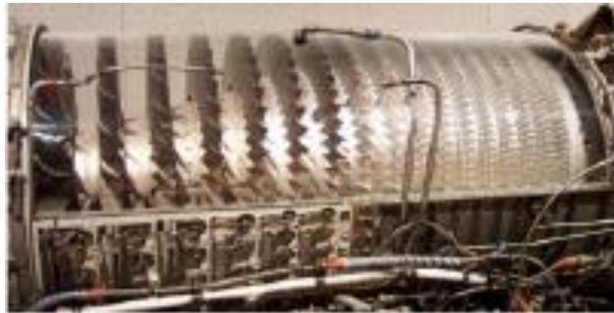
Figure 1.18 – Boro-aluminum fan blades of the first and third stages in engine J-79
