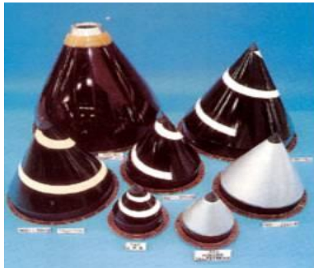
Figure 1.15 – Rolls-Royce fan nose spinners
