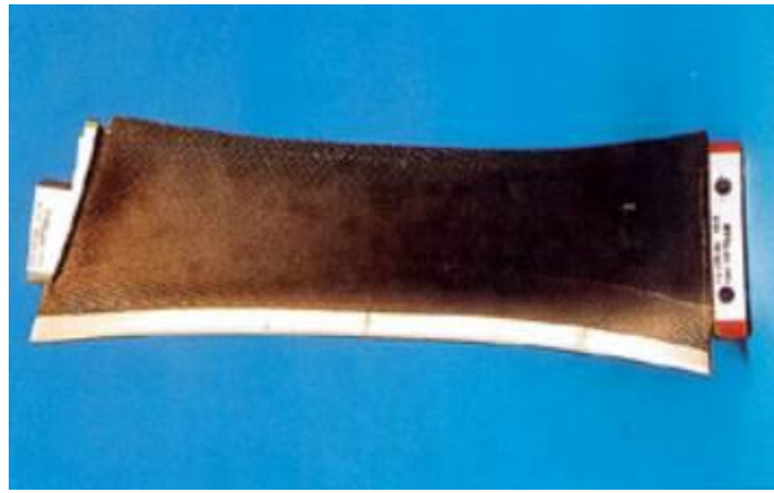
Figure 1.16 – A carbon fibre reinforced epoxy Trent fan outlet guide vane
