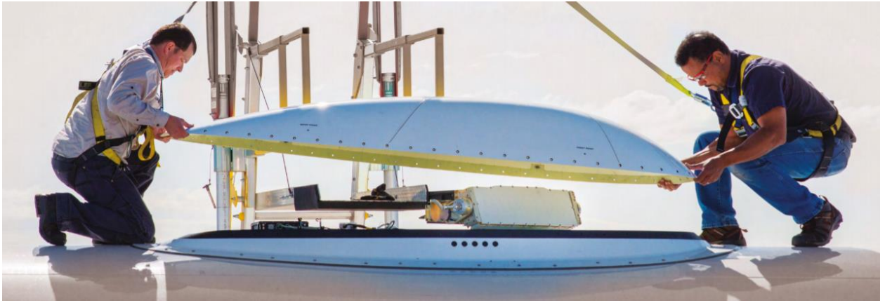
Рисунок 2.2.4.1 Installation of fuselage antenna and radome
