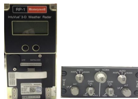
Fig. 3.14. Receiver-transmitter and control panel of SSJ-100 WXR
