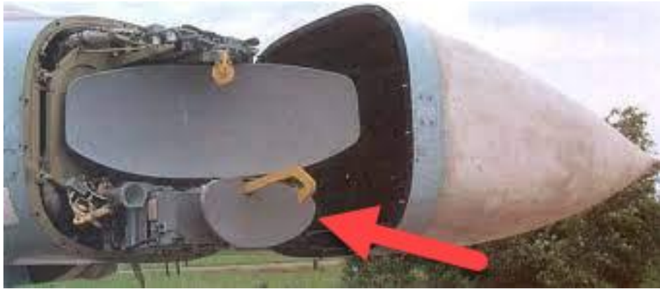
Fig. 3.9 . Radar of profile flight "Relief"
