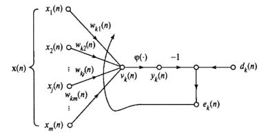
Figure 1.2 Illustration of the neuron signal transmission graph
