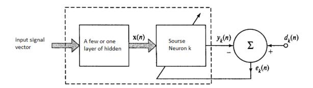
Figure 1.1 Block diagram for the output node of the neural network
