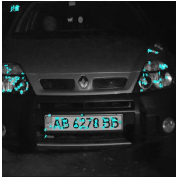
Fig. 4.34. The results of the detection of characteristic points at close to minimum permissible level of artificial lighting
