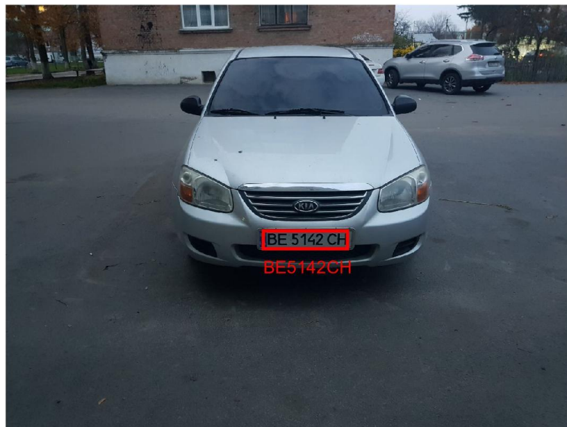
Fig. 4.32. System operation at the minimum daytime level of illumination
