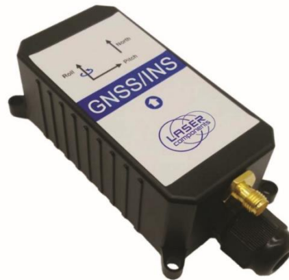
Fig. 1.10 - Integrated navigation system based on MEMS components BW-GI100/200
