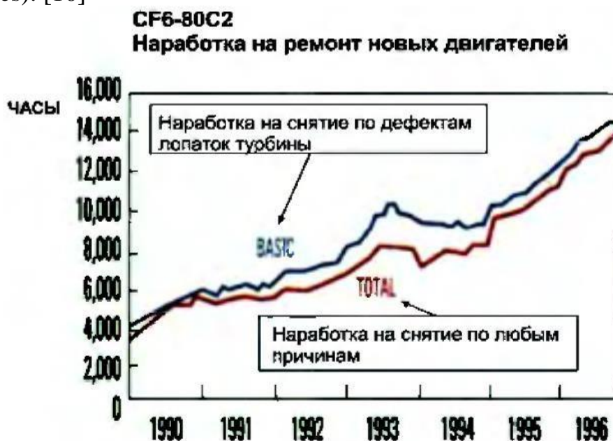
Figure 2.1 - Average MTBF of new CF6-80C2 engines on removal from wing - by turbine blade defects and by all defects taken together on "removal from wing" due to turbine blade failure, by all defects [12]
