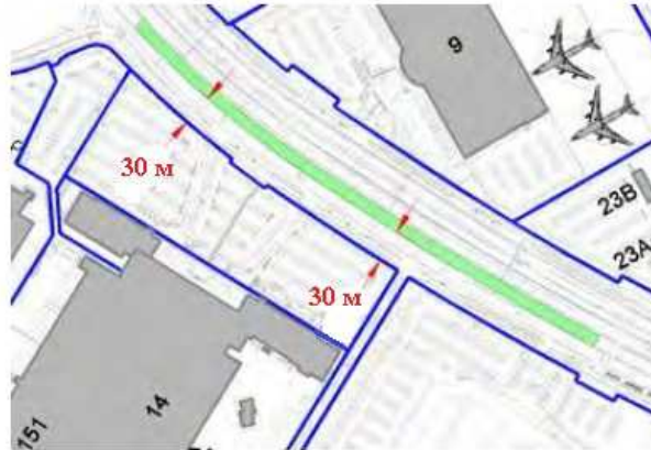
Figure 2. Restrictions on the lines of the internal transport connections, which are not the main approach roads to an airport
