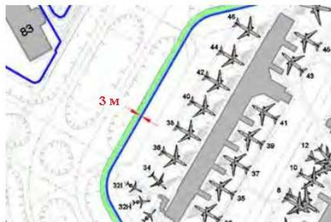
Figure 5. Restrictions on the lines of the internal engineering-service connections of an airport [10]
