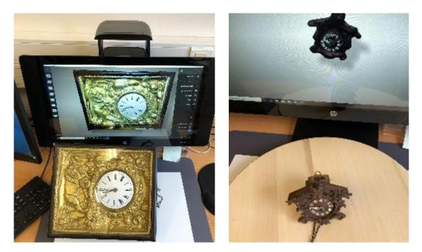
Figure 2: HP Sprout Pro G2 digitization process. During digitization it is necessary to rotate the object manually. The resulting model and its comparison can be seen in the picture. Left - a problem with larger clocks that are shiny and have a glass lid.
