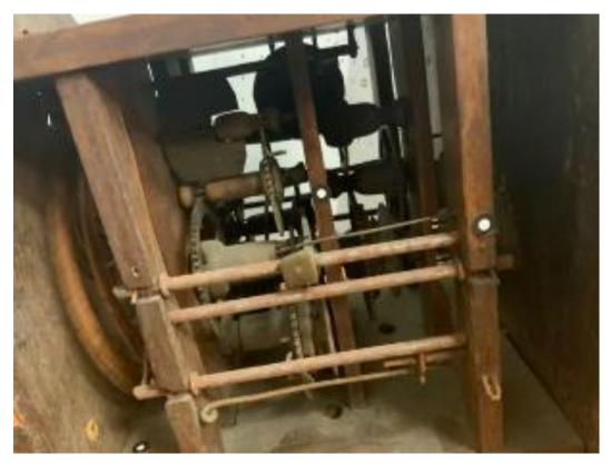
**Figure 1**: Example of a clock that has an exposed clock machine. The visible black and white dots are reference points. Some types of scanners use them to focus on a digitized object in space. In this case it is used by the ATOS Compact Scan 2M measuring device
