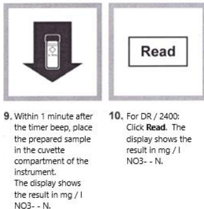
Fig. 2.7. Nitrate testing procedure on spectrophotometer (part 3)
