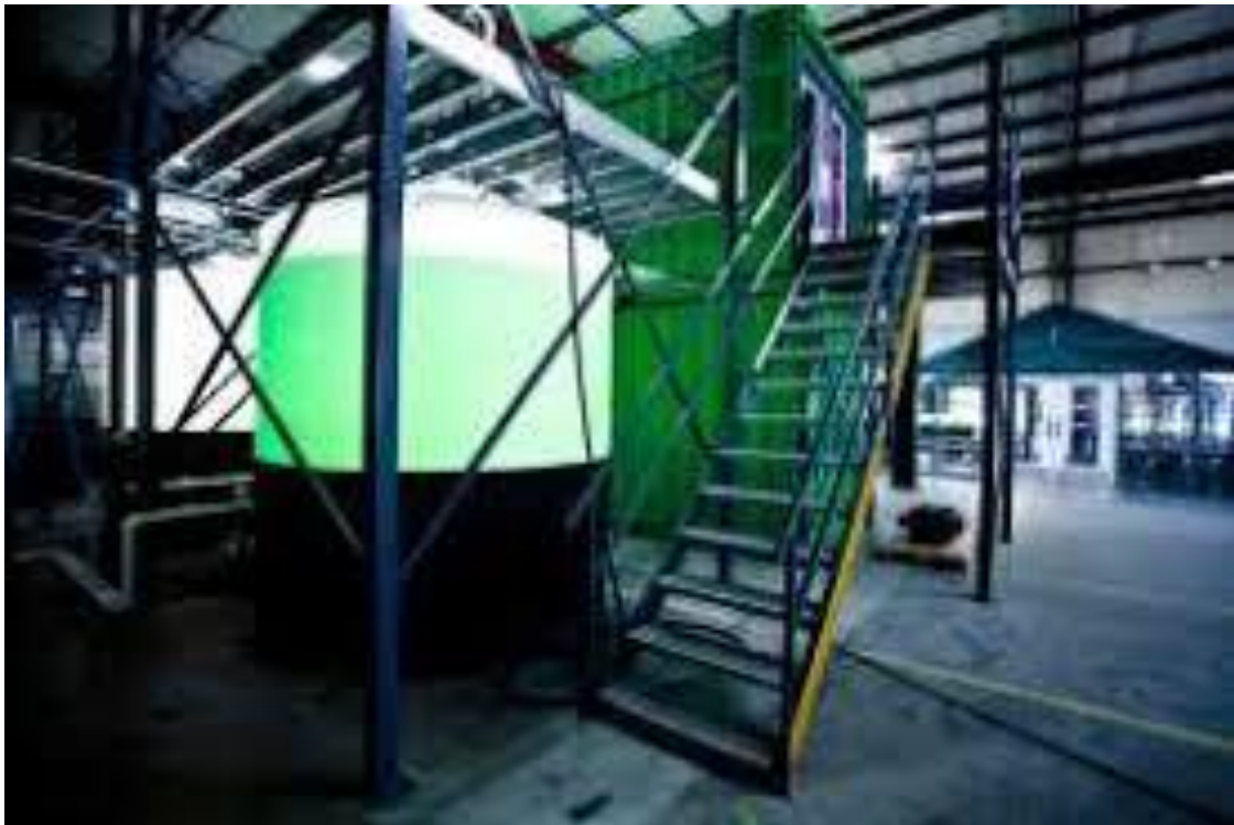
Figure 2.5. Photobioreactor for algae biomass cultivation, Algae Extraction and Processing Center (Atlanta, USA)
