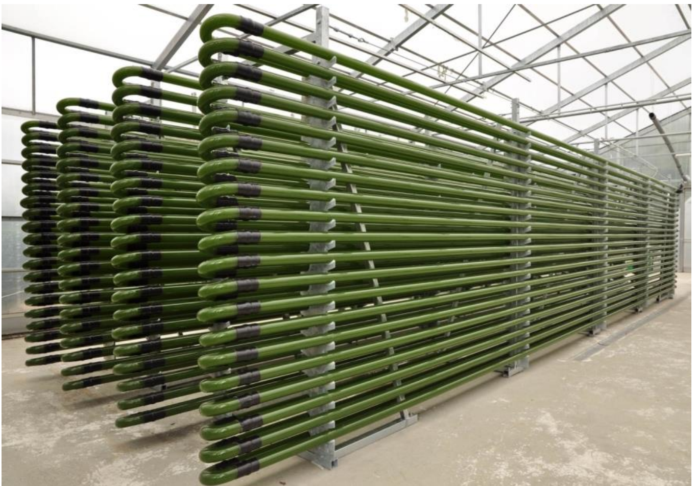
Fig. 2.4. Closed algae biomass cultivation systems
