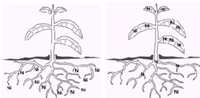
Fig.1.1. Uptake of metals Ni by phytoextraction. Nickel is removed from soil by moving up into plant roots, stems, and leaves. The plant is then harvested and disposed of and the site replanted until the Ni in the soil is lowered to acceptable levels.
