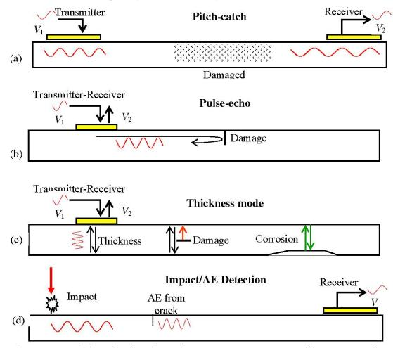
Figure 3.33 - Functional process of the piezoelectric wafer active sensors
