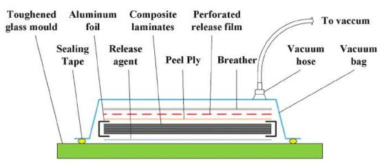
Figure 1.11 - Vacuum bagging fabrication method
