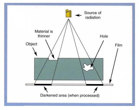
5) It requires access to both sides of the test object.
