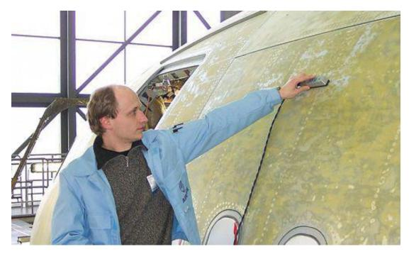
Figure 2.22 - Eddy current inspection carried out on the fuselage
