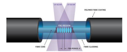
Figure 3.30 - Fiber optic sensor representation
