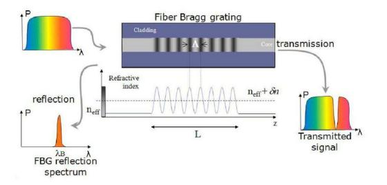
Figure 3.31 - Fiber Bragg grating principle of operation
