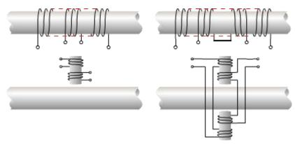
Figure 2.23 - Representation of the absolute mode of operation
