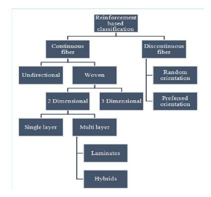
Figure 1.5 - Classification of fiber reinforcement
