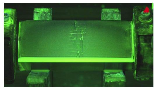
Figure 2.19 - Magnetic particle fluorescent inspection
