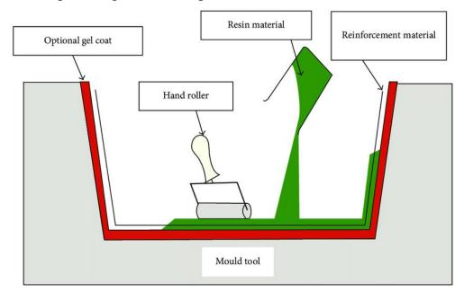
Figure 1.12 - Hand layup fabrication technique
