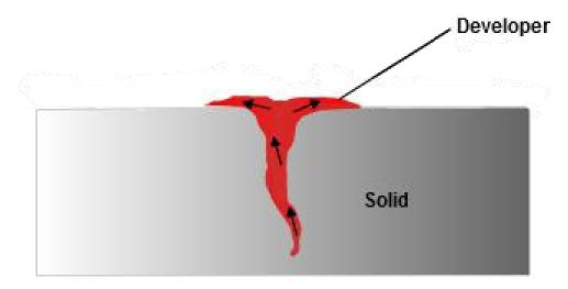
Figure 2.20 - Representation liquid penetrant inspection technique
