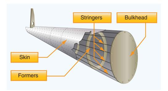
Figure 1.2 - Semi monocoque fuselage configuration
