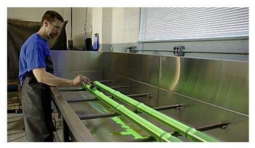
Figure 2.21 - Fluorescent liquid penetrant inspection
