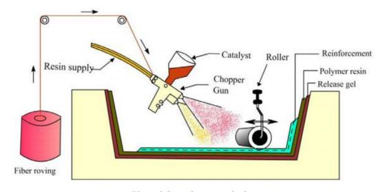
Figure 1.9 - Spray layup fabrication method
