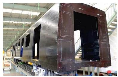
Figure 1.8 - Train made of carbon fiber
