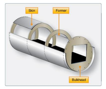
Figure 1.1 - Monocoque fuselage configuration
