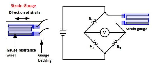
a) Strain gauge b) strain gauge functional diagram Figure 3.35 - The representation electrical strain gauge
