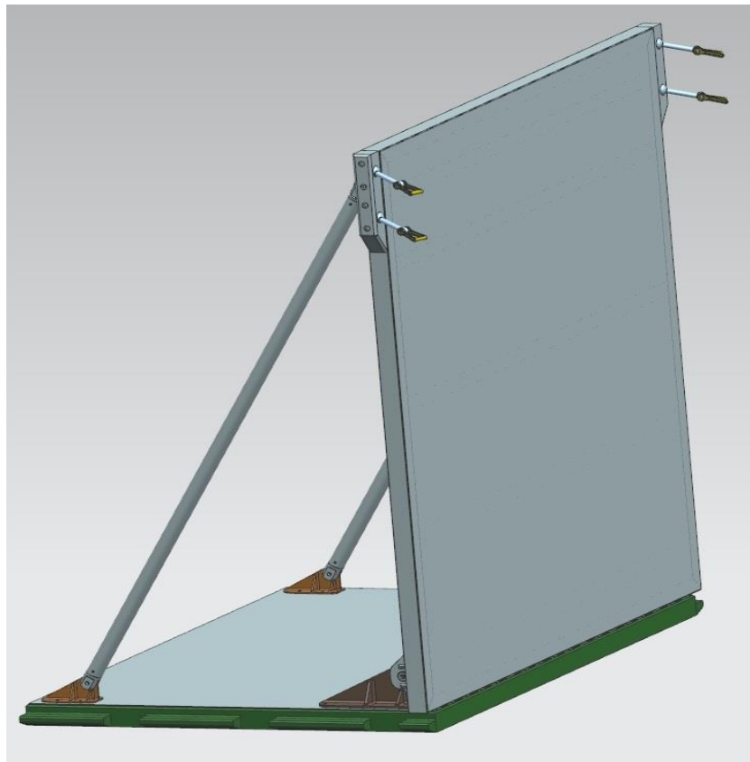
Figure 4.14 – General view of buffer stop
