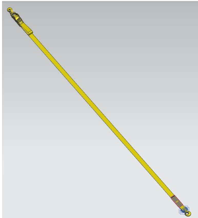
Figure 4.13 - General view of the mooring belt
