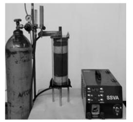
Figure 3. High-temperature unit for thermal treatment of carbon materials by TMEC
