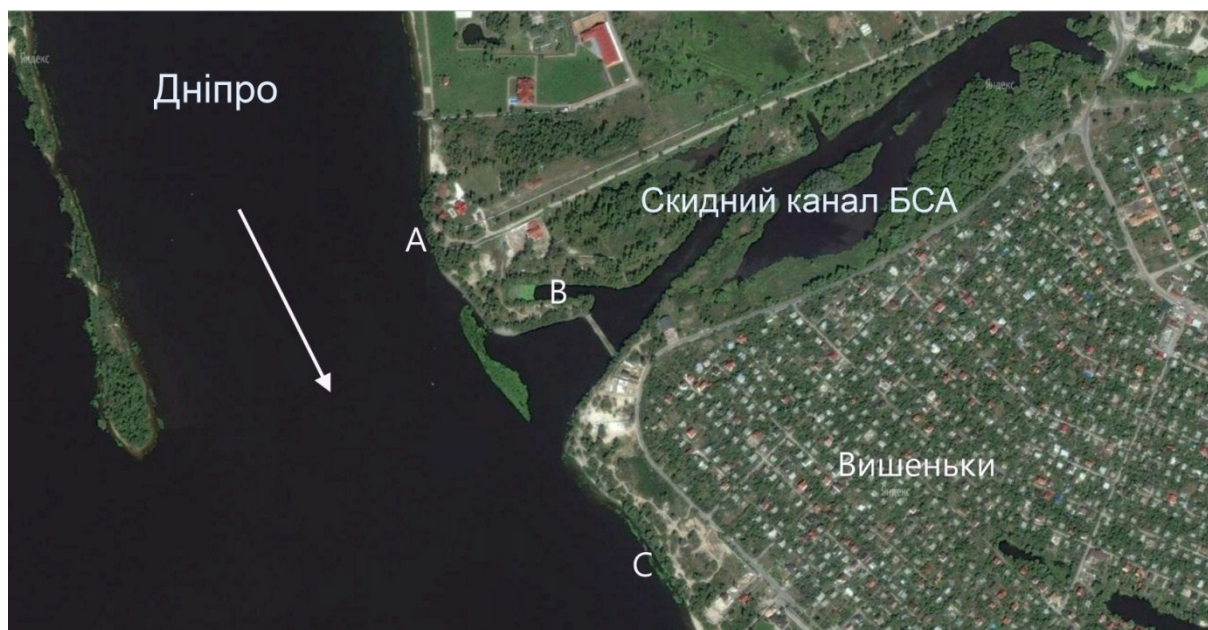
Fig. 2.2. Map-scheme of water water sampling in the area of discharge of Bortnytsia aeration station: A - above the discharge into the Dnieper 200 m; B - discharge channel BSA; C - below the discharge into the Dnieper 250 m.
