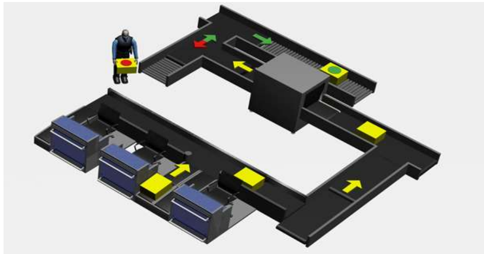
Fig. 1.5 Installation for 150 units baggage / hour
