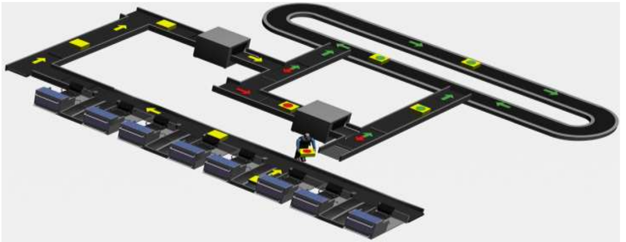
Fig. 1.3 Installation for 600 units baggage / hour
