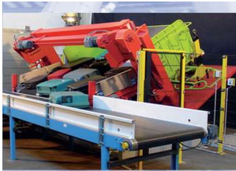
Fig. 2.4 Mechanical unloading module
