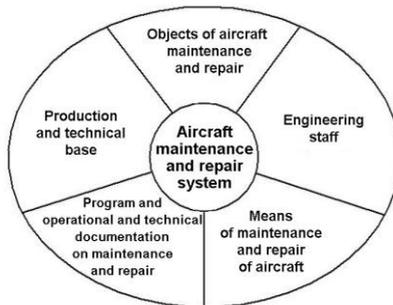
Fig. 3. The generalized structure of the aircraft maintenance and repair system
