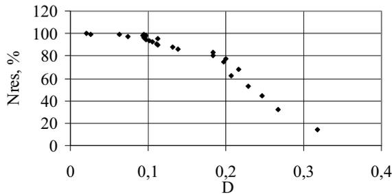
Fig. 4. Relationship between residual life and damage parameter  $D$ .
