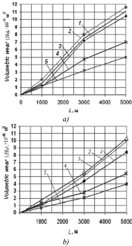
**Fig. 2.** The dependence of volumetric wear value from the friction path during the study of anti-wear properties of a basic TS-1 jet fuel (a) and TS-1 jet fuel (b) processed with electric field for one hour at voltage  $U = 2000$  V and a field strength  $E = 1,1 \cdot 10^6$  V/m at a normal load  $P = 10$  kg: 1 -  $g = 0.550$  m/s; 2 -  $g = 0.847$  m/s; 3 -  $g = 1.38$  m/s, 4 -  $g = 2.196$  m/s, 5 -  $g = 3.36$  m/s
