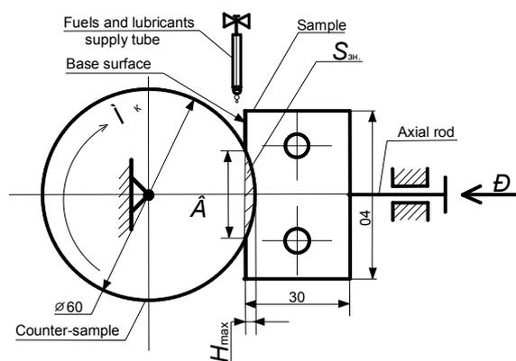
**Fig. 1.** A scheme of testing of anti-wear properties of fuels and lubricants, implemented on the "PT-4TS" friction device
