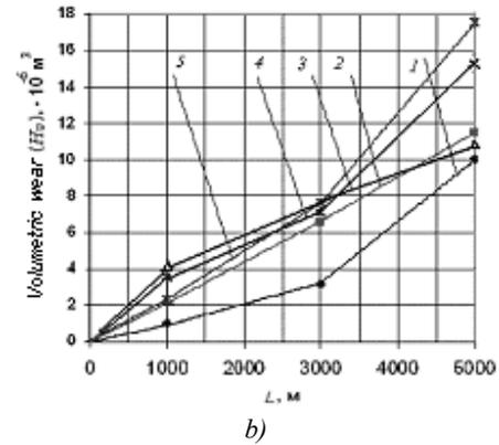
**Fig. 3.** The dependence of volumetric wear value from the friction path during the study of anti-wear properties of a basic TS-1 jet fuel (a) and TS-1 jet fuel (b) processed with electric field for one hour at voltage  $U = 2000$  V and a field strength  $E = 1,1 \cdot 10^6$  V/m at a sliding speed  $g = 0,847$  m/s: 1 -  $P = 10$  kg; 2 -  $P = 15$  kg; 3 -  $P = 20$  kg; 4 -  $P = 25$  kg; 5 -  $P = 30$  kg
