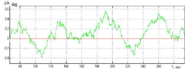
Fig. 10. The results of simulation of gyro-accelerometric method in case of navigation complex operation in aerometric mode
