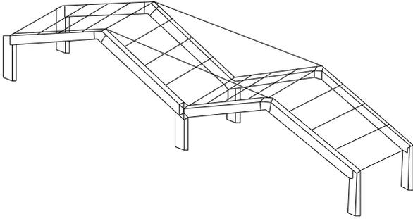
Fig.6. Frame of multispan skeleton building with straining beam
