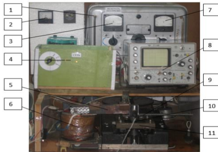
Fig. 1. Equipment for research of materials on friction and wear during reverse movement: 1 – an independent power source for creating a magnetic field in the friction zone, 2 – ammeter for recording the magnetic field, 3 – ammeter for recording the current in the friction zone, 4 – chopper, 5 – magnetic circuit, 6 – inductor, 7 – power source, 8 – an oscilloscope for recording the parameters of the electric current in the magnetic circuit, 9 – loading, 10 – friction knot, 11 – capacity for the working medium.
