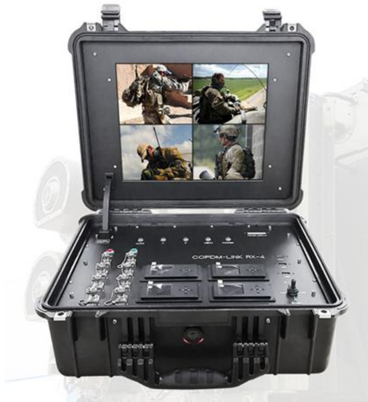
Рис. 2.3 Portable Ground Control Station(GCS) For UAV, UGV
