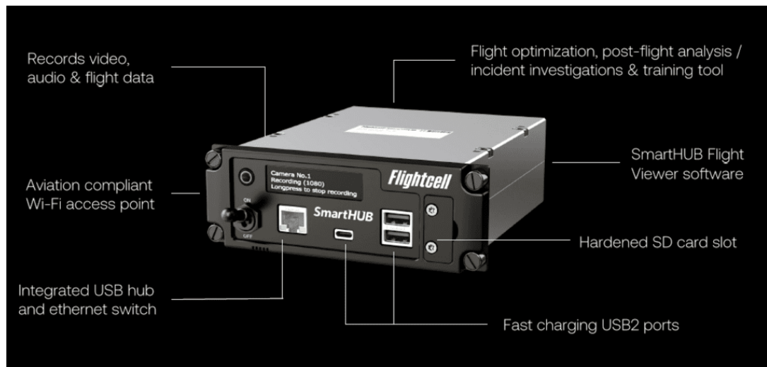
Fig.1.15. Flightcell's new SmartHub is an HD video, audio, flight data recorder and access point for USB/IP devices. (Flight cell)
