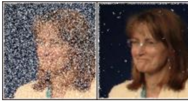
Figure 3.1. Use of a median filter to improve an image severely corrupted by defective pixels
