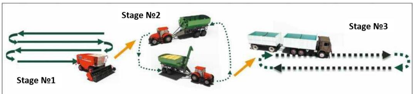
Fig. 3.3 The three-stage grain harvesting "Combine - Bunker-transloader PBN-30 – MAN TGX with semi-trailer Bodex KIS 3WA"
