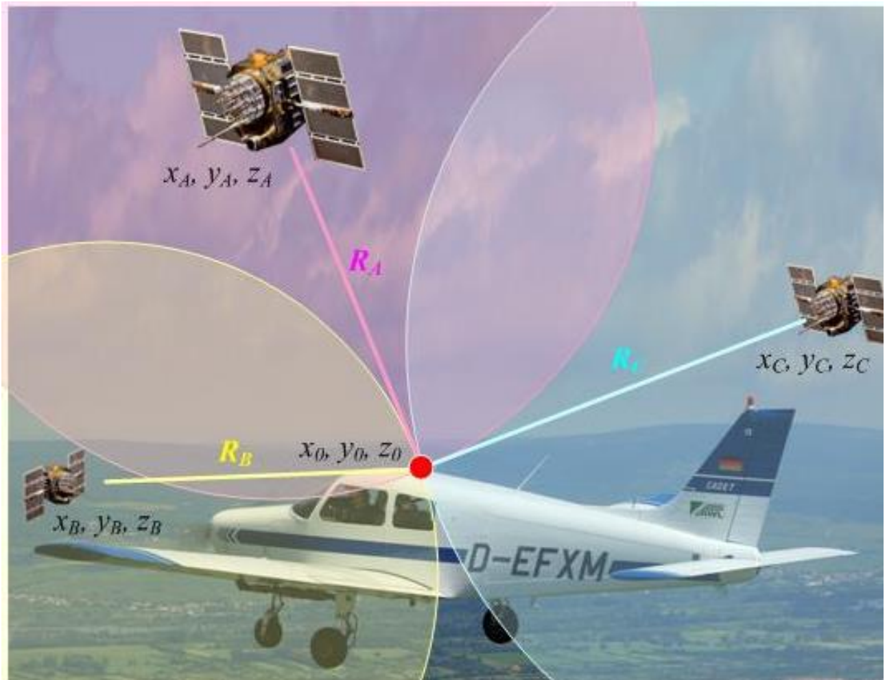
Figure 1.2 – Principle of obtaining aircraft coordinates by GNSS [58]
