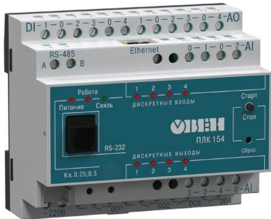
Figure 4. Programmable logic controller
