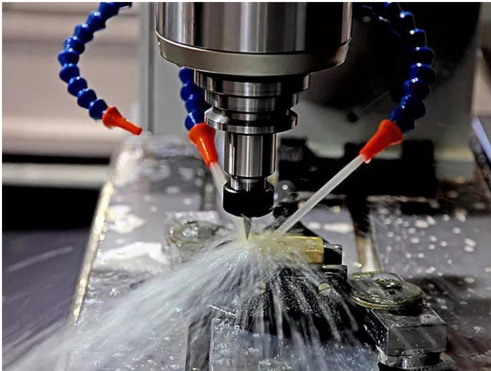
Figure 5.1 Cutting fluid during cutting process
