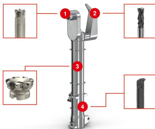
Figure 1.14 Cutting tools to machine the main cylinder
