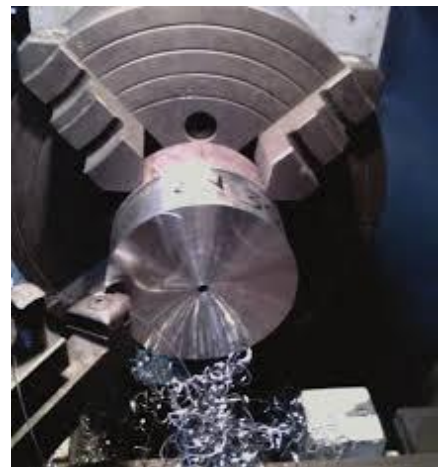
Figure 3.2 - Scheme of tests of cutting tools at continuous increasing the cutting speed
