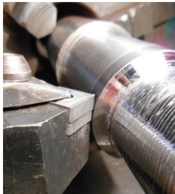
Figure 3.4 - The position of the insert relative to the processed part in determining the resistance to failure and wear under contact load on lathes
