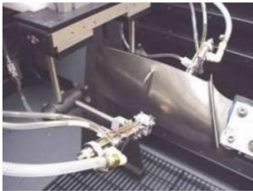
Figure 1.7 - Laser shock peening and damage tolerance data of F101 engine first fan blade
