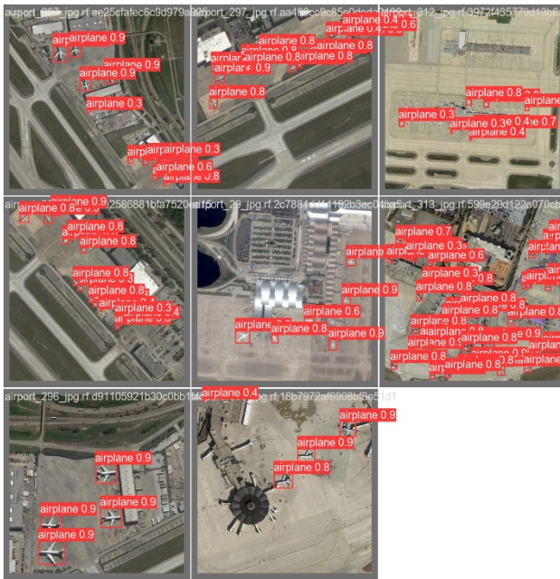
Fig. 3. Visualization of airplane detection and classification
