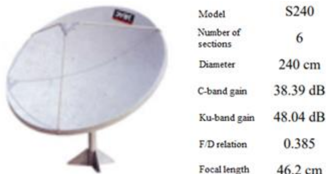
Fig. 3.3 Appearance antenna and its technical characteristics
