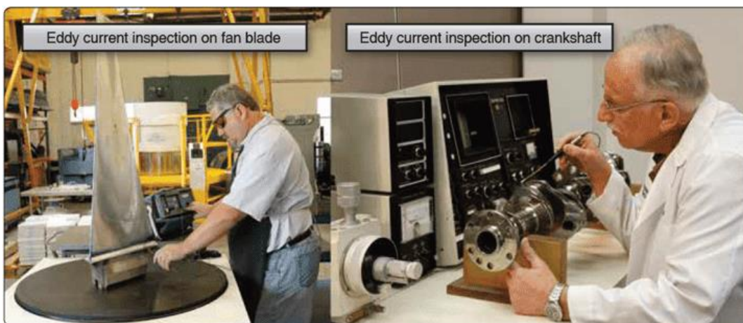
Figure 1.4 Eddy's current inspection
