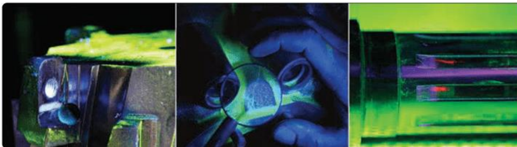
Figure 1.3 Dye penetrant inspection
