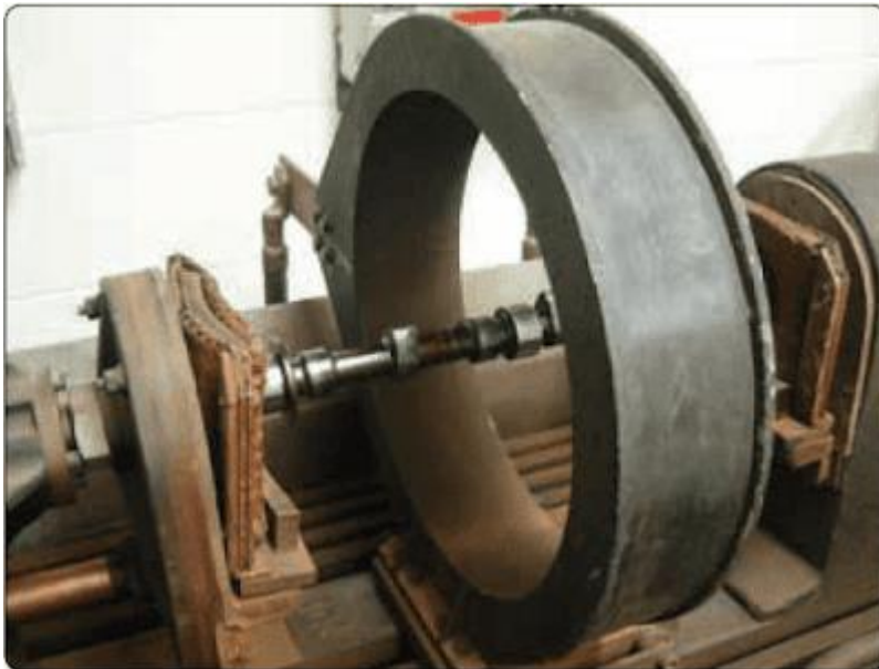
Figure 1.24 Longitudinal magnetization of camshaft (solenoid method)
