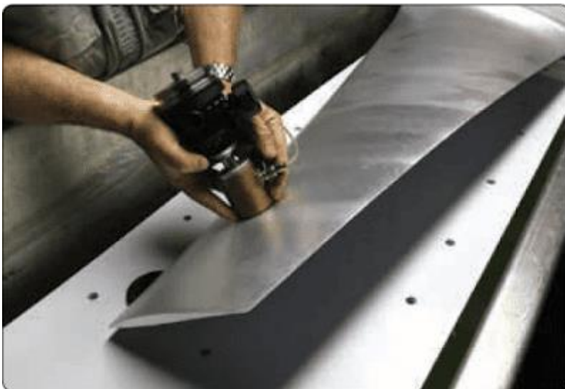
Figure 1.19 Ultrasonic inspection of a composite structure
