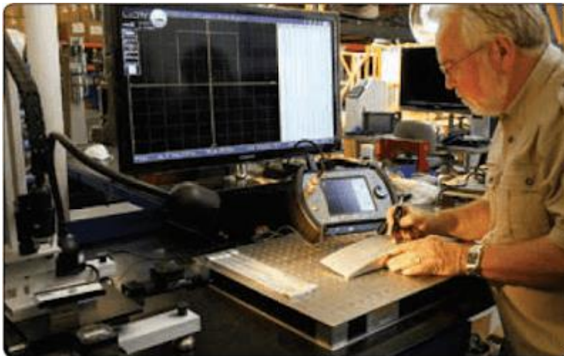
Figure 1.7 Impedance plane test
