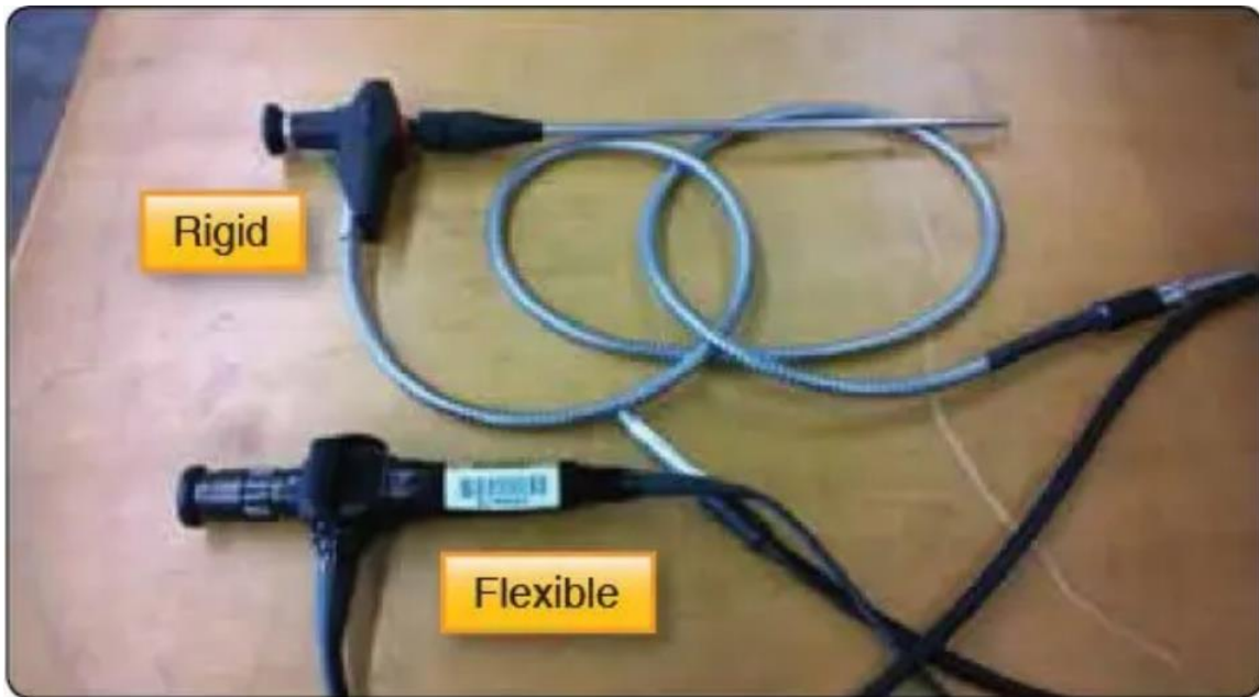
Figure 1.2 Rigid and flexible borescopes
