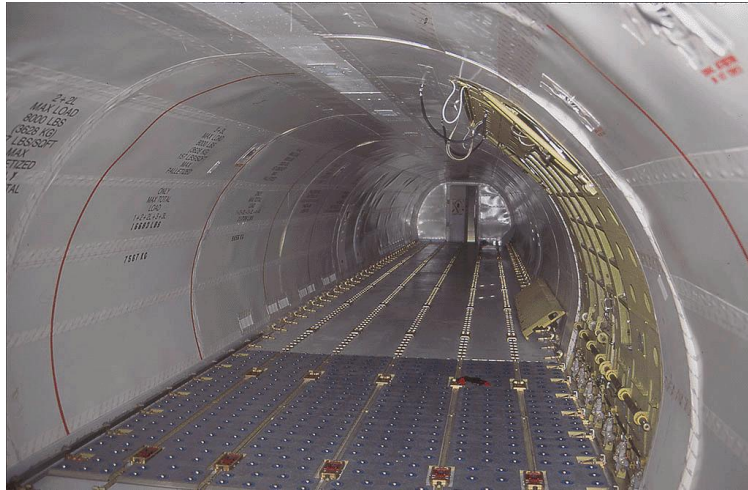
Fig.2.3 - Ball Mats of the plane A321, selected as a prototype in the preliminary design procedure (part 1)
