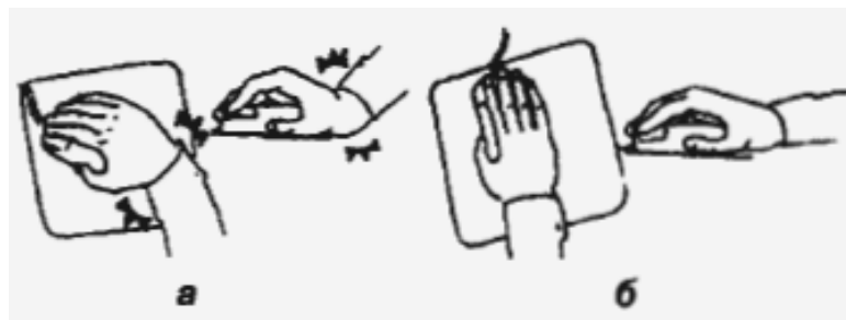
Fig. 3.2. The position of the hand and forearm when working with device type "mouse": a - incorrect; b – correct.
