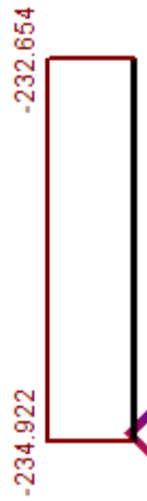
Figure 3.14– Column with the largest internal value efforts N under the 1st type of load
