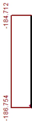
Figure 3.19– Column with the largest internal value efforts N under the 6th type of load
