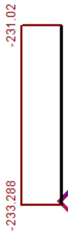
Figure 3.15– Column with the largest internal value efforts N under the 2nd type of load
