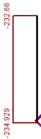
Figure 3.16– Column with the largest internal value efforts N under the 3rd type of load
