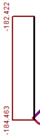
Figure 3.21– Column with the largest internal value efforts N under the 8th type of load
