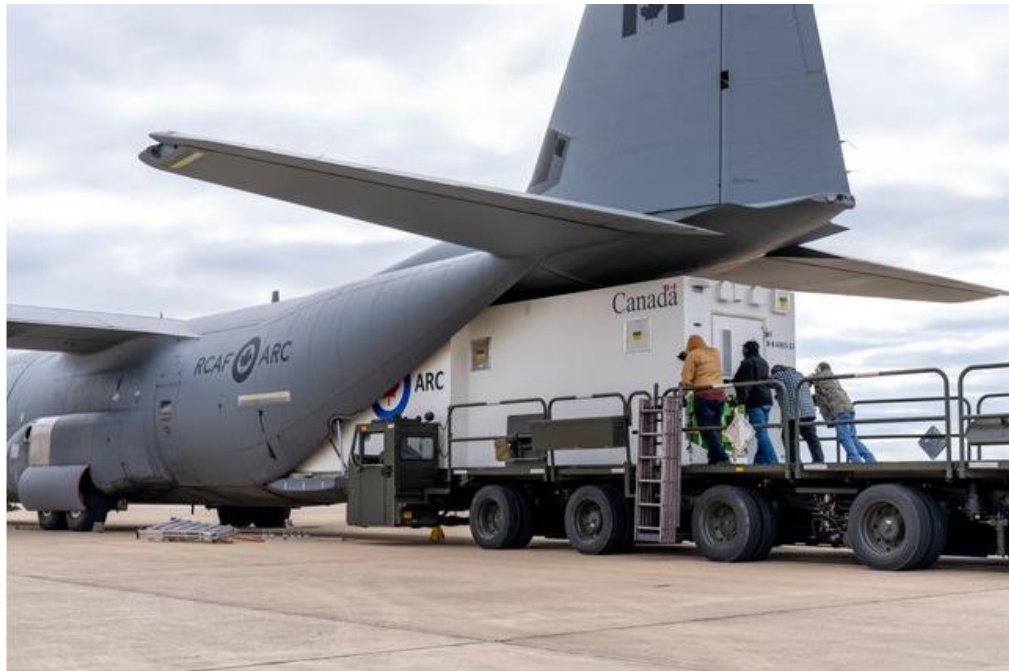
Figure 2.3. – Installation of medical module
