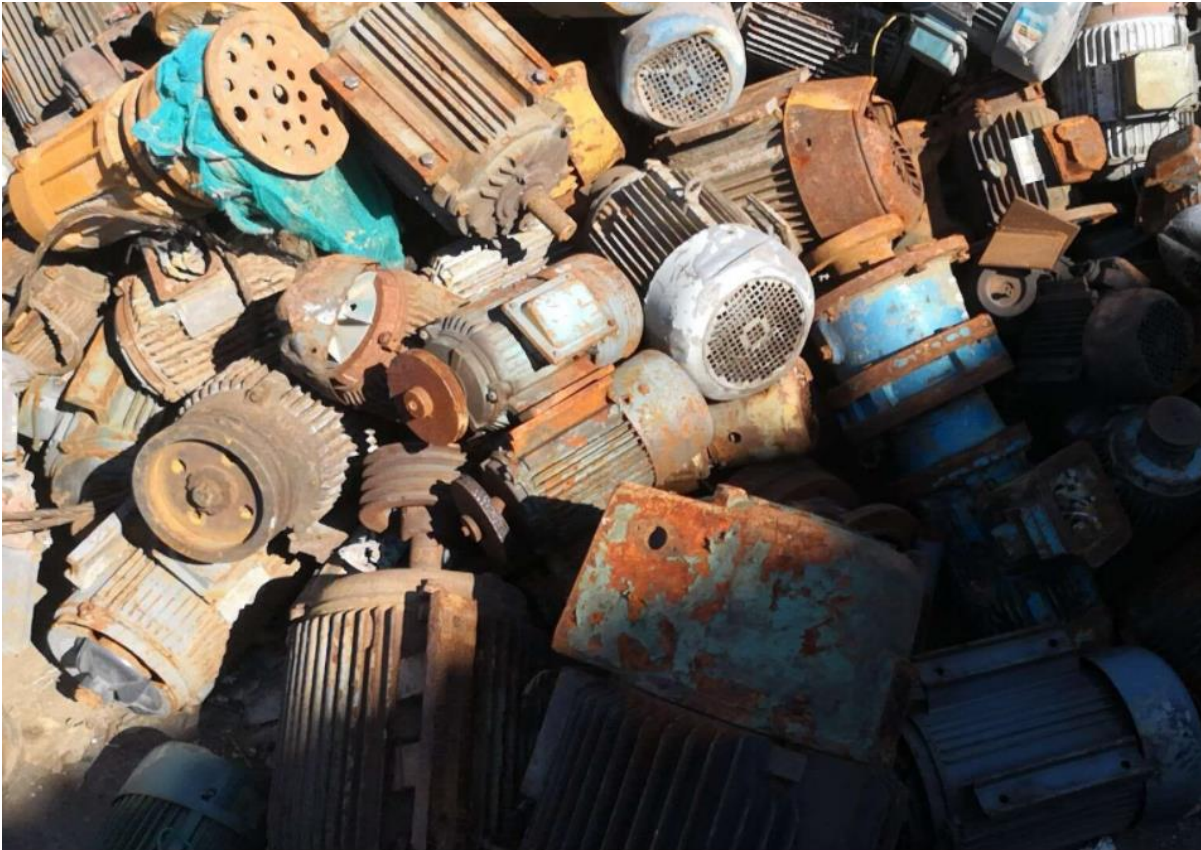
Fig. 1.5 – Electrical motor corrosion.
