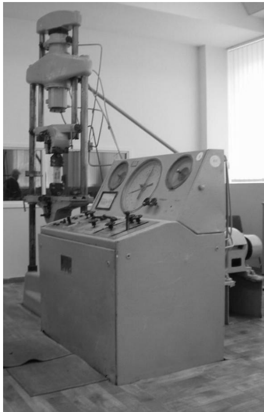
Fig. 2.6 – Fatigue test machine for the investigation negative side effects of CPC application
