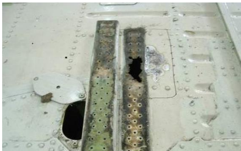
Fig. 1.8 - Due to the high possibility of moisture accumulation, the longitudinal beams (stringers) of the fuselage were corroded
